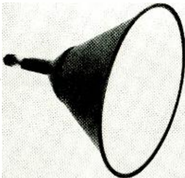
Fig. 1—The 19AP4, a large-screen picture tube used in many 1951 receivers.
